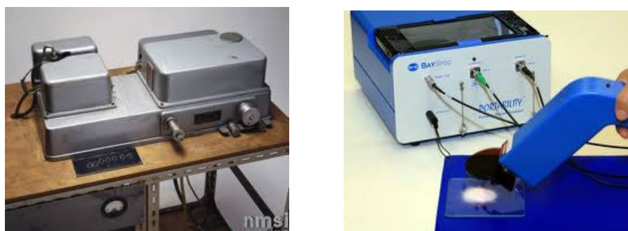
Figure 1 – a) Dispersive IR spectrometer 1968 b) In-field Raman spectrometer 2010
